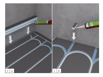
In wet areas, the open ends of the groove in the edge areas of the wedi PreLine must be waterproof.
